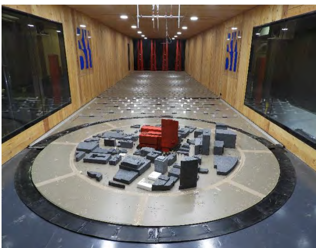
Image 2c: Wind tunnel study model – Existing + All Office Final Development Plan configuration
