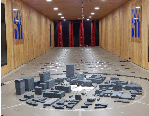
Image 2a: Wind tunnel study model - Existing configuration
