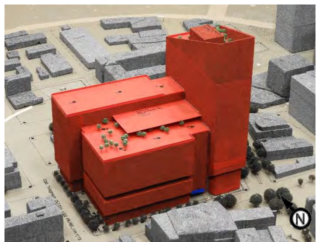
Image 2c: Wind tunnel study model – Existing + All Office Final Development Plan configuration
