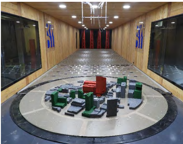
Image 2e: Wind tunnel study model - All Office Final Development Plan + Cumulative configuration
