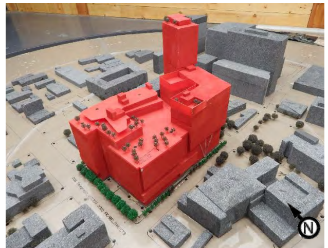
Image 2b: Wind tunnel study model – Existing + Residential/Office Mix Final Development Plan configuration
