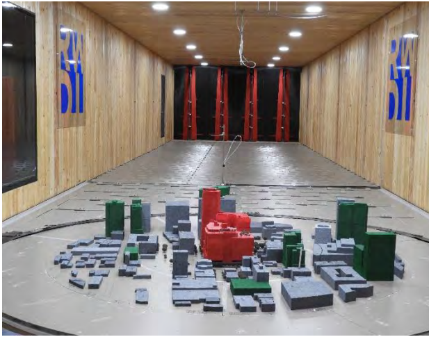
Image 2d: Wind tunnel study model - Residential/Office Mix Final Development Plan + Cumulative configuration
