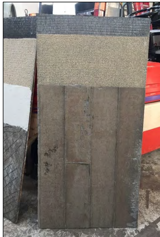
Image 17: View of the mockup of the mortared finish that would be applied over the CFRP wrap to resemble the existing board-formed-finish. Source: BCA, Inc. January 2017.
