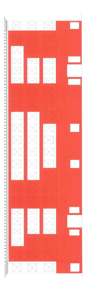
54% OF FACADE COVERED BY SHOTCRETE (UPPER LEVELS ONLY) 65% OF FACADE COVERED BY SHOTCRETE (ALL LEVELS)
