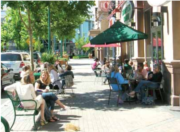
The functional zones of the public sidewalk include a building frontage zone, an amenity zone, and a pedestrian zone. (DG 139)
