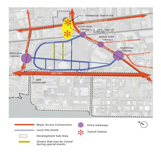
Figure 5.1: Sub-Area A Street Circulation Diagram
