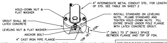
INSTALL STANDARD ON LEVELING NUTS. PLUMB STANDARD AND TIGHTEN HOLD-DOWN NUTS. FILL ENTIRE SPACE UNDER POLE FLANGE WITH LATEX CONCRETE GROUT.
