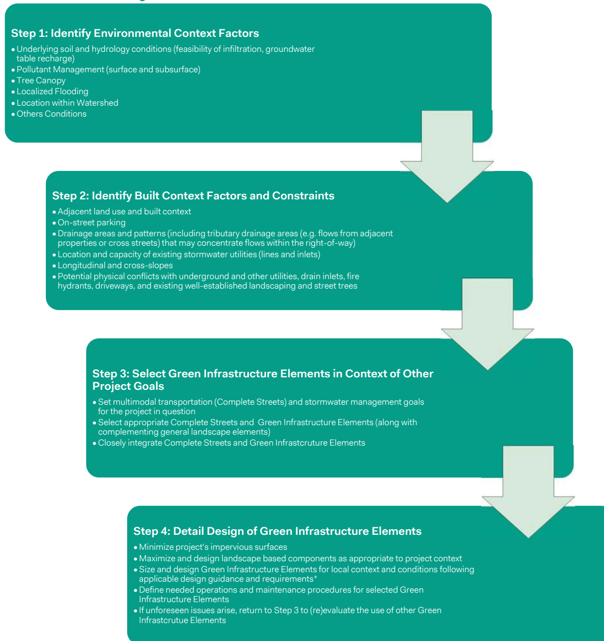
Figure 5-1. Green Infrastructure in Street Design Process
